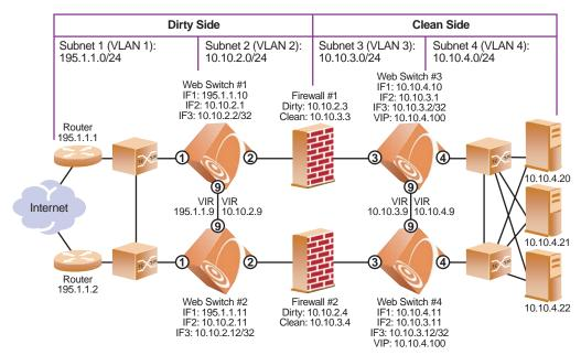
Figure 13-7 Four-Subnet FWLB Example Network
